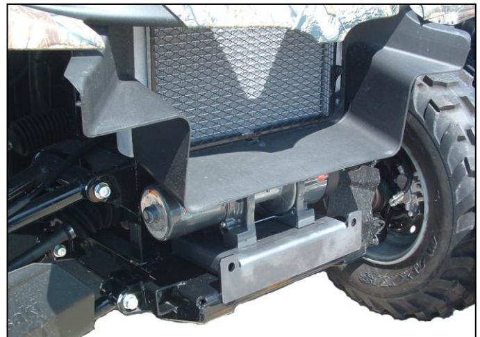
"Figure 5" Winch Mount Assembly in Position
